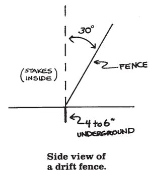
**Figure 1:** A funnel trap with a drift fence can be used to capture rattlesnakes. Adapted from Byford (1983).
